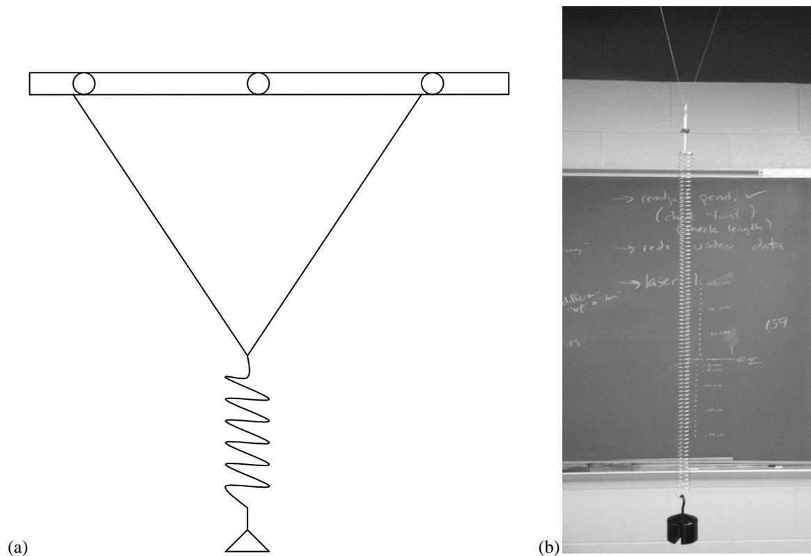
**Figure 1.2:** *The sketch (a) is not to scale. The total length of the system ended up being about 1.6 meters, which is why I could only include the lower portion in the photo (b). Also, these images both show the string fixed at two points rather than just one as previously indicated; this discrepancy will be explained in the next section. I used a hooked weight as the pendulum “bob.”*
