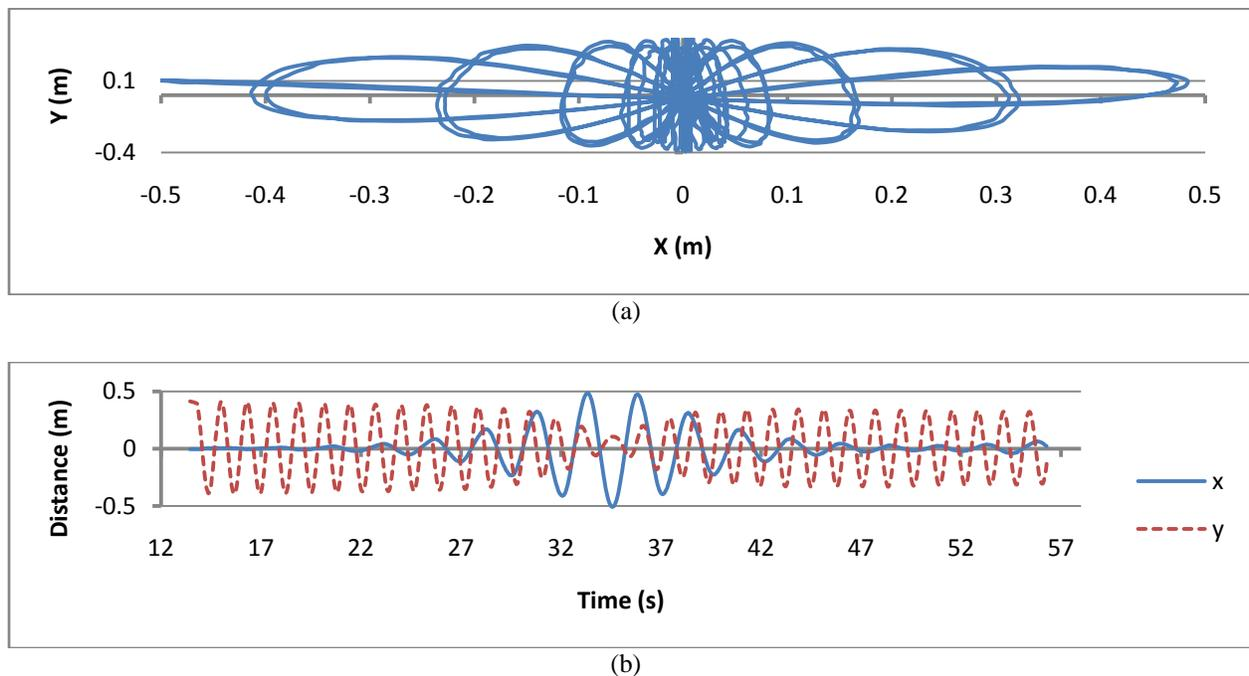
**Figure 3.4:** These graphs show (a) the  $x$ - $y$  behavior and (b) the time evolution of the coordinates for the Butterfly Mode. Notice how the near perfect symmetry of (b) highlights the constant change in the phase relationship between the pendulum and spring frequencies.
