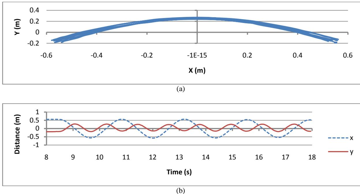
**Figure 3.1:** *These graphs indicate (a) the x-y behavior as well as (b) the time evolution of the coordinates for the Concave Down Parabolic Mode. Notice that there are multiple parabolic paths due to damping in the system. Also, we can see here that the x and y behavior are in step with each other due to the phase lock of the pendulum and spring oscillations.*
