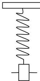
**Figure 1.1:** *A rough sketch of a Wilberforce pendulum. The vanes trace figure-eights as a result of the system's two degrees of freedom.*
