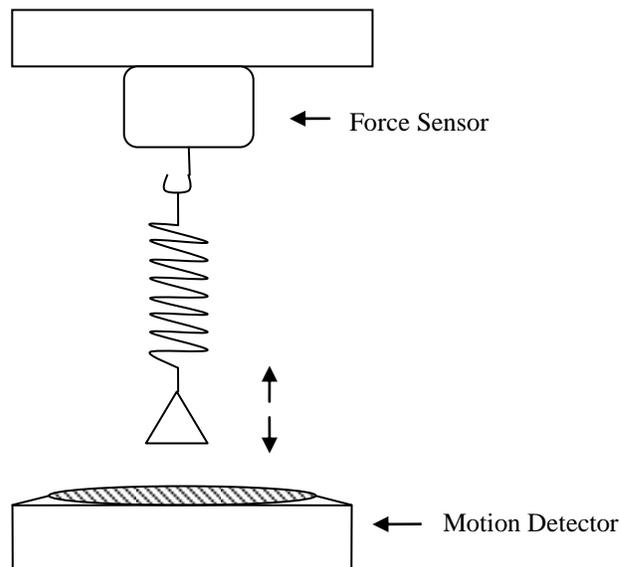
**Figure 1.3:** This is a diagram of the setup for determining the spring constants of the springs.
