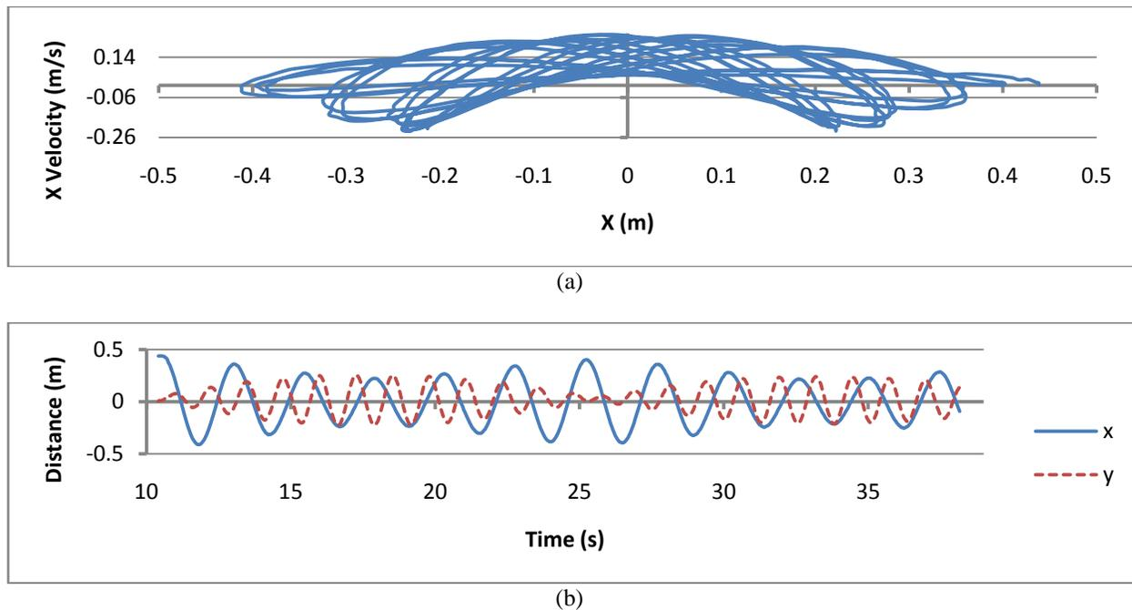
**Figure 3.3:** (a) illustrates the  $x$  and  $y$  behavior of the Indeterminate Mode with a Concave Down Parabola, while (b) shows the time evolution of the coordinates for this mode. It is evident from (b) that the phase relationship between the pendulum and spring frequencies is not constant.
