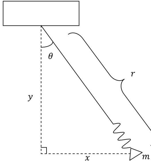
**Figure 2.1:** This figure represents a still of the pendulum in motion. The variables  $x$  and  $y$  can be represented in terms of  $r$  and  $\theta$  using the properties of a right triangle.
