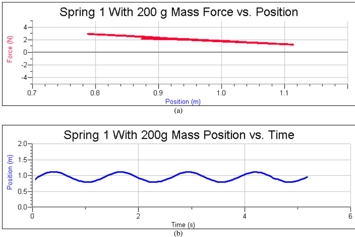
**Figure 1.4:** *These graphs illustrate (a) force with respect to position for Spring 1 and (b) position with respect to time for Spring 1 with a 200g mass. The slope of the line in (a) is equal to the negative of the spring constant of Spring 1, while (b) shows that the period of this spring/mass system is just over 1 second long.*
